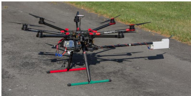
Figure 2: DJI S-1000 is 41" diagonally and weighs 9.25 lbs.
